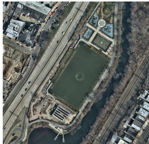
In the WEDG-certified Starlight Park project, a continuous 12-foot-wide, shared-use greenway path winds along both sides of the Bronx river and is connected by four new bicycle/pedestrian bridges.
