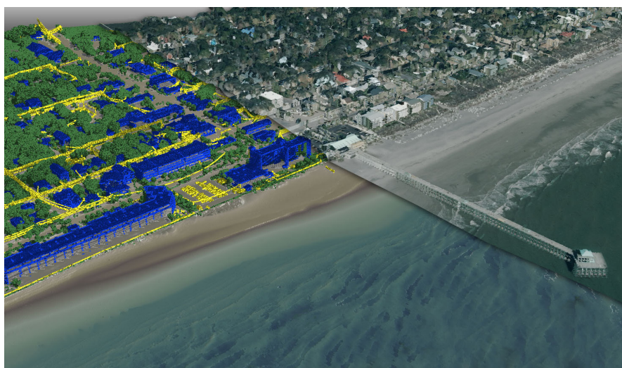
Split view of the North Carolina shoreline showing the above-ground lidar point cloud colored by classification (left) and imagery right) overlaying the bare earth model (bottom)
