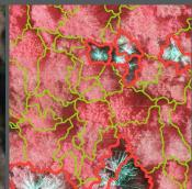
Transmission cage clearance zones identifying vegetation encroachments for a lattice tower (left). Segmented vegetation crown polygons are created from lidar point cloud geometries. CIR photos are falsely colored to display near infrared as red. Bright tones represent healthy vegetation producing chlorophyll, an unhealthy tree is distinct (right).
